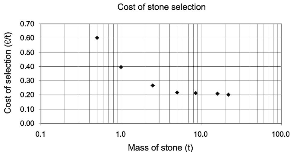
**Figure 3.89** Estimation of the cost associated with selecting different armourstone sizes. Costs in euros. The differences result after combining the increased cost of the greater hydraulic excavator capacity needed and the speed of working expressed in terms of total tonnes selected per hour (courtesy J van Meulen)
