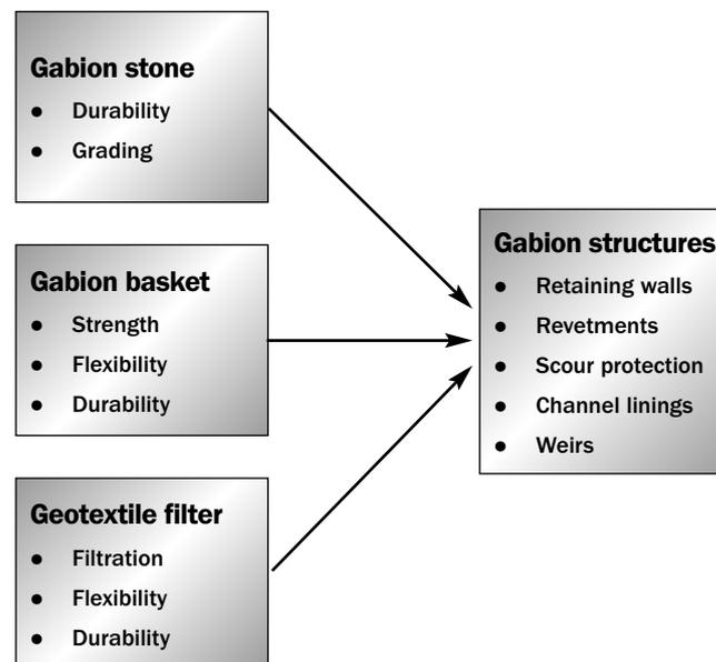
**Figure 3.102** Key features and applications of gabion structures
