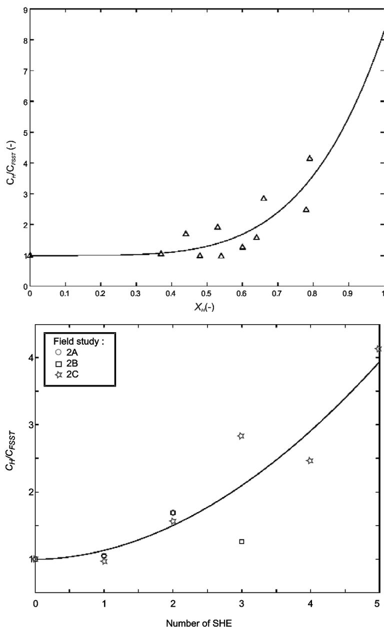
**Figure 3.37** Variation of integrity as determined with the FSST with repeated standardised rough handling events; Top: as a function of  $X_H$ . Bottom: as a function of the number of handling events (SHE). A fourfold increase in integrity is seen after between four and six handling events
