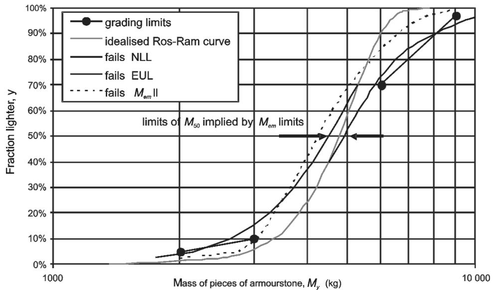
**Figure 3.21** Illustration of compliance and non-compliance with the grading system requirements for a 3–6 t standard grading
