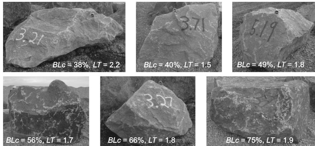
**Figure 3.17** Comparison of shape parameters of heavy armourstone, where increase in blockiness does not always correspond with increase or decrease in value of *LT* (mass shown in tonnes) (courtesy S Newberry)
