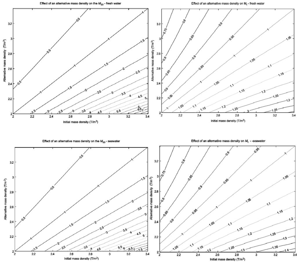
**Figure 3.29** Contour plots of multiplication factors for change in density. Top: Fresh water,  $\rho_w = 1.0$  t/m<sup>3</sup>; bottom: Seawater,  $\rho_w = 1.025$  t/m<sup>3</sup>
