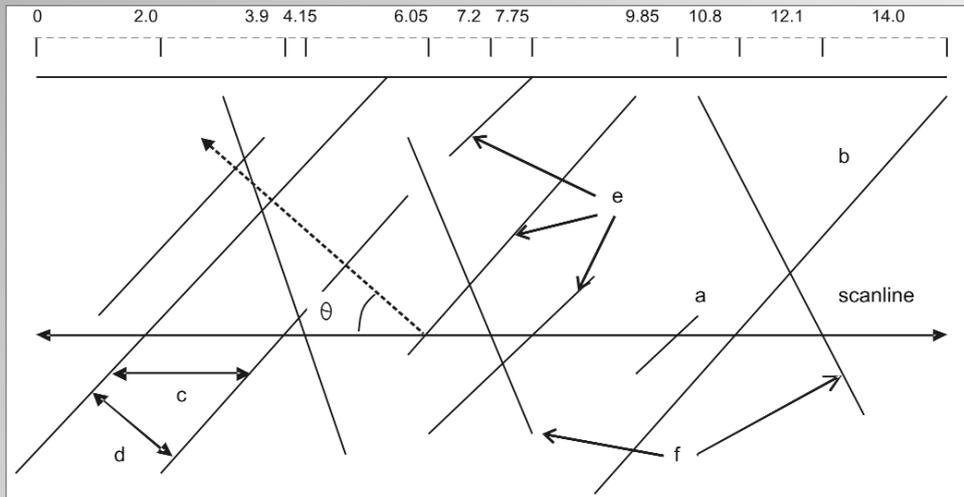
**Figure 3.50** Scanline mapping showing spacing between discontinuity sets and example measurements. a: non-persistent discontinuity: length < 3 m; b: persistent discontinuity: length ≥ 3 m; c: spacing (DS); d: principal spacing (PS); e: Set A; f: Set B;  $\theta$  is the angle between the scanline and a line normal to a discontinuity set.
