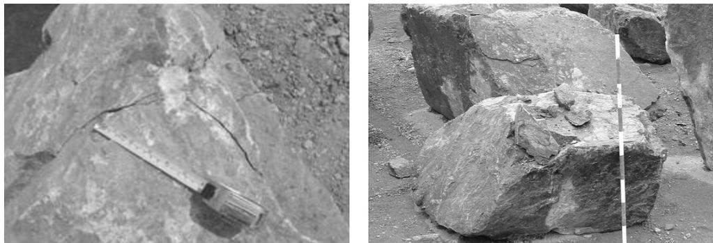
**Figure 3.11** Examples of minor breakage taking place in sedimentary and igneous rock (courtesy S Dupray)
