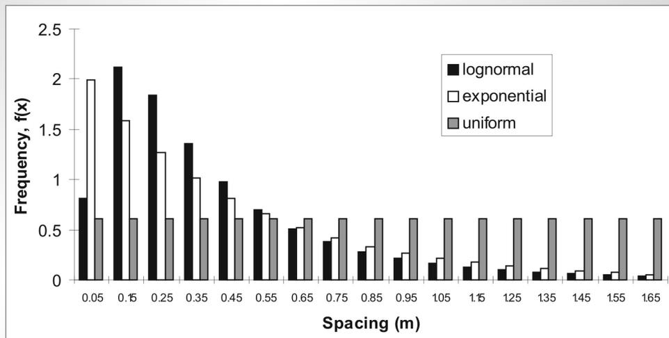
**Figure 3.52** Illustration of three commonly found principal spacing distributions for discontinuity sets
