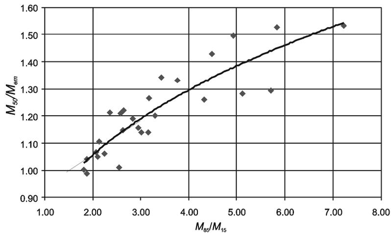
**Figure 3.22**  $M_{50}/M_{em}$  as a function of the grading width,  $M_{85}/M_{15}$ , measured from field project data (see Equation 3.16) (on the basis of investigations carried out by J A van Meulen)
