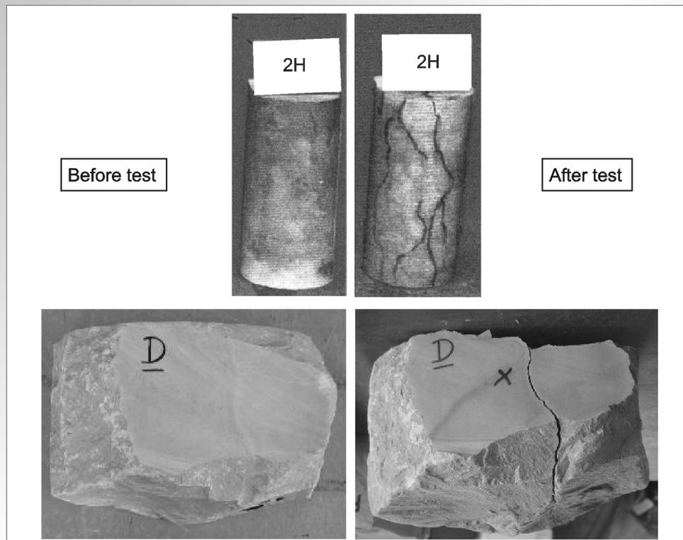
**Figure 3.46** Samples before and after freeze-thaw test using sonic velocity. Top: specimen with wet surface displaying discontinuities and significant decrease of sonic velocity after test. Bottom: specimen displaying open cracks and significant decrease of sonic velocity. Before test: Sonic velocity,  $V_p = 5100$  m/s, continuity index,  $I_c = 76$  per cent; after test:  $V_p = 2600$  m/s,  $I_c = 40$  per cent (Top: courtesy S Dupray, bottom: courtesy J Perrier, CNR)
