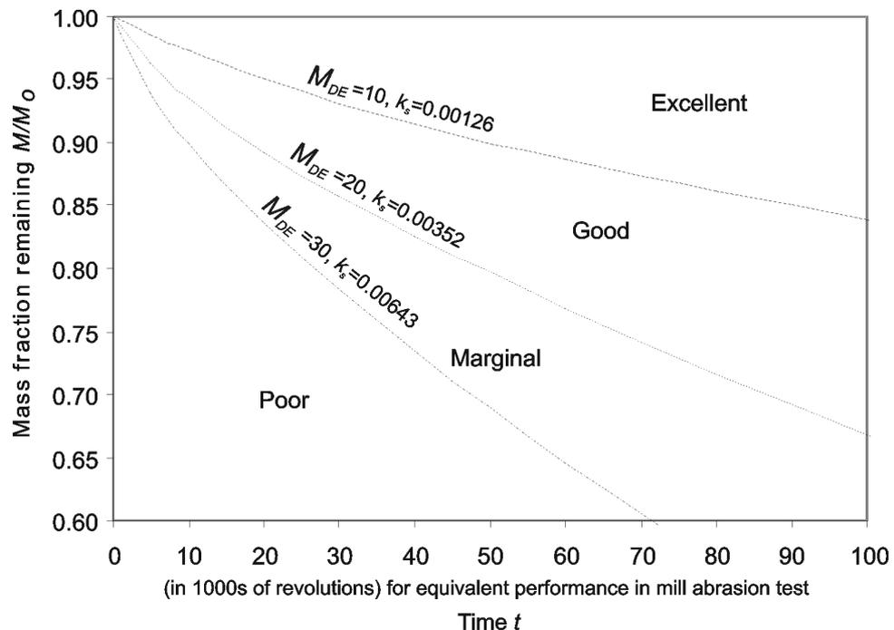
**Figure 3.30** Abrasion resistance classification chart based on Micro-Deval test results.  $M_{DE}$  values have been converted using Equations 3.36 and 3.37 to mass loss plots indicative of the equivalent mill abrasion test results. The quality boundaries for abrasion resistance have been revised from earlier published positions for compatibility with the European standard  $M_{DE}$  specification categories (courtesy J van Meulen)
