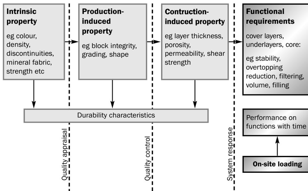
**Figure 3.4** Conceptual scheme for material properties and functions, illustrated for armourstone
