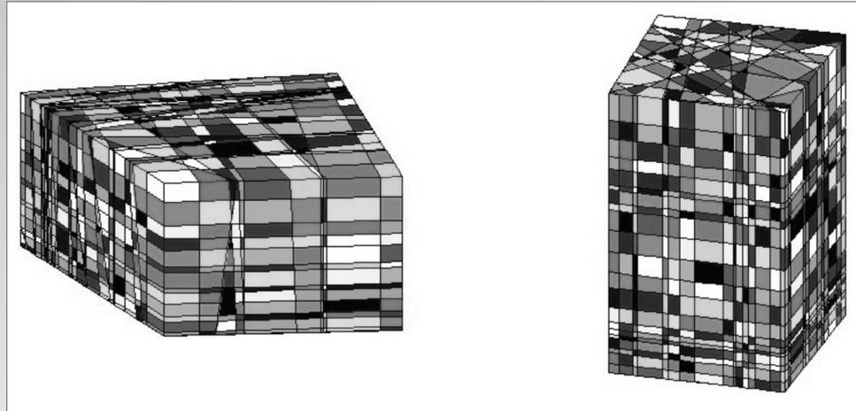
**Figure 3.60** Computational dissection of rock masses – left: from Zone B (2100 m<sup>3</sup>); right: Zone D (975 m<sup>3</sup>) – using discontinuity location and orientation data from three perpendicular scanline segments
