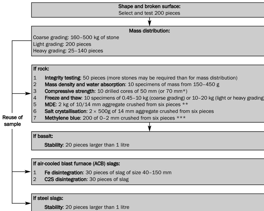
**Figure 3.39** Sampling chart identifying possible multiple uses of the same samples and test pieces leading to economies in the testing programme
