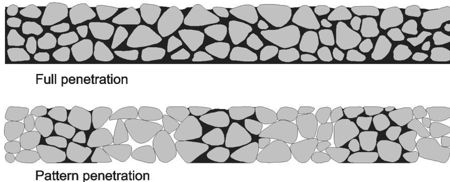
**Figure 3.109** Grout penetration methods for a rock revetment
