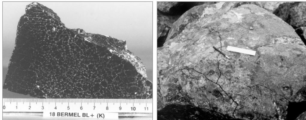
**Figure 3.47** Stones affected by the “Sonnenbrand effect” (courtesy G Laan). Left: pattern on the surface of basalt rock, leading to severe failure; right: considerable cracking interpreted as being caused primarily by Sonnenbrand effects
