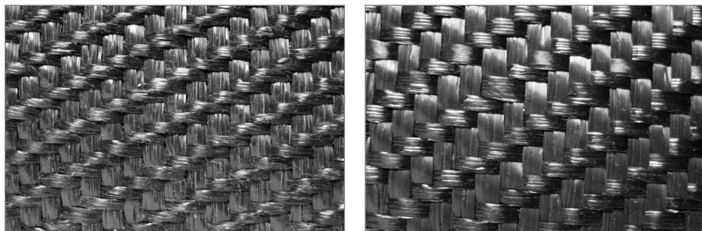
**Figure 3.111** *Woven geotextiles (courtesy Ten Cate)*
