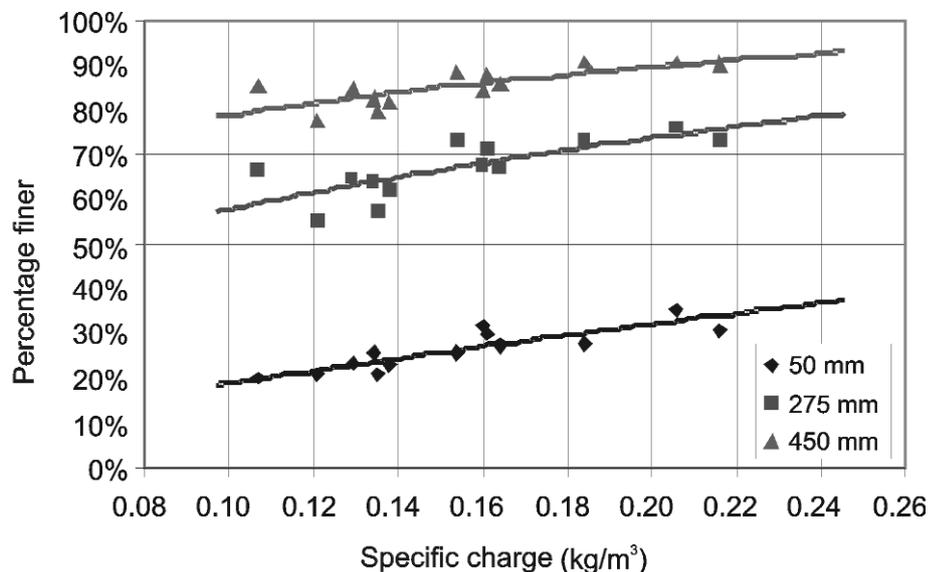
**Figure 3.57** Use of a three-point method to characterise fragmentation and demonstrate the decrease in  $D_{150}$  with increasing specific charge of ANFO – data from one quarry (courtesy J van Meulen)
