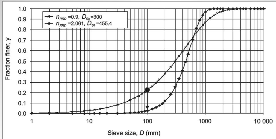
**Figure 3.24** Illustration of change in size distribution resulting from fines removal below 1 kg and limiting of oversize blocks
