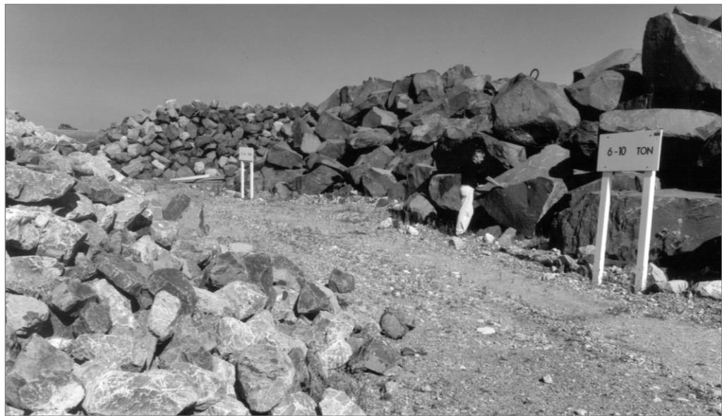
**Figure 3.66** *Armourstone organised in several standard grading stockpiles*
