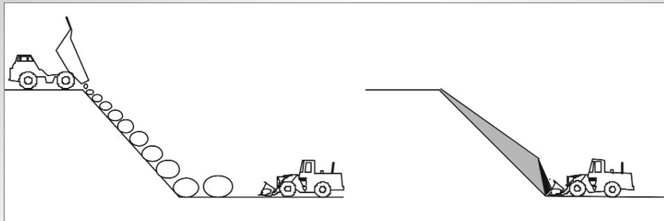
**WARNING:** safe procedure is to dump first and then doze over the side, not direct tipping as is shown.
