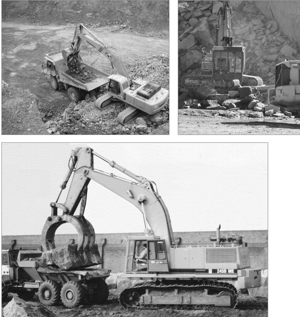
**Figure 3.78** Use of excavator for handling. Top left: mounted on tracks clearing muckpile and sorting oversize (courtesy S Dupray); top right: mounted on track with grid bucket selecting stones after secondary breakage with hydraulic hammer (or pecker) (courtesy S Dupray); bottom: with high-capacity five-tine power fork at the quarry for individual handling of heavy stones (courtesy J van Meulen)
