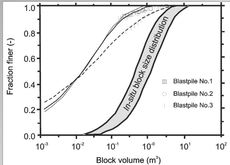
**Figure 3.59** *In situ and blastpile armourstone size distributions determined from photo-scanline and oversize stockpile measurements from three different blast designs in a limestone quarry. Lines based on linking oversize with photo-scanline determination of  $D_{b63.2}$*
