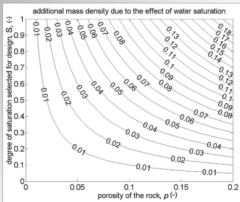
**Figure 3.9** Effect of degree of saturation  $S_r$  (-), on the apparent mass density of porous rock  $\rho_{app}$ . Contours indicate the correction value (in  $t/m^3$ ) to be added to the dry mass density  $\rho_{rock}$
