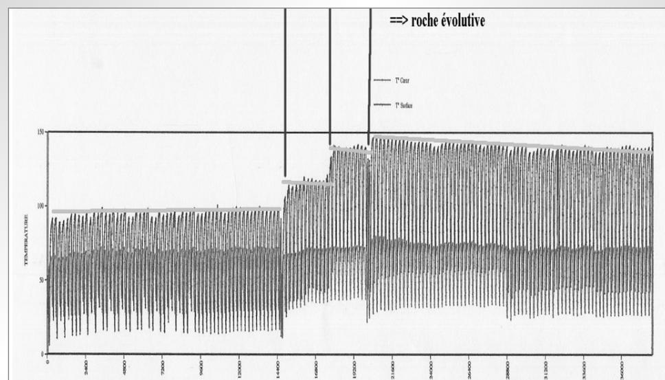
**Figure 3.48** Trace recording of thermal cycling. The lower trace indicates the inside temperature, the upper trace the surface temperature; the steps reveal the rock has undergone degradation (courtesy J Perrier, CNR)
