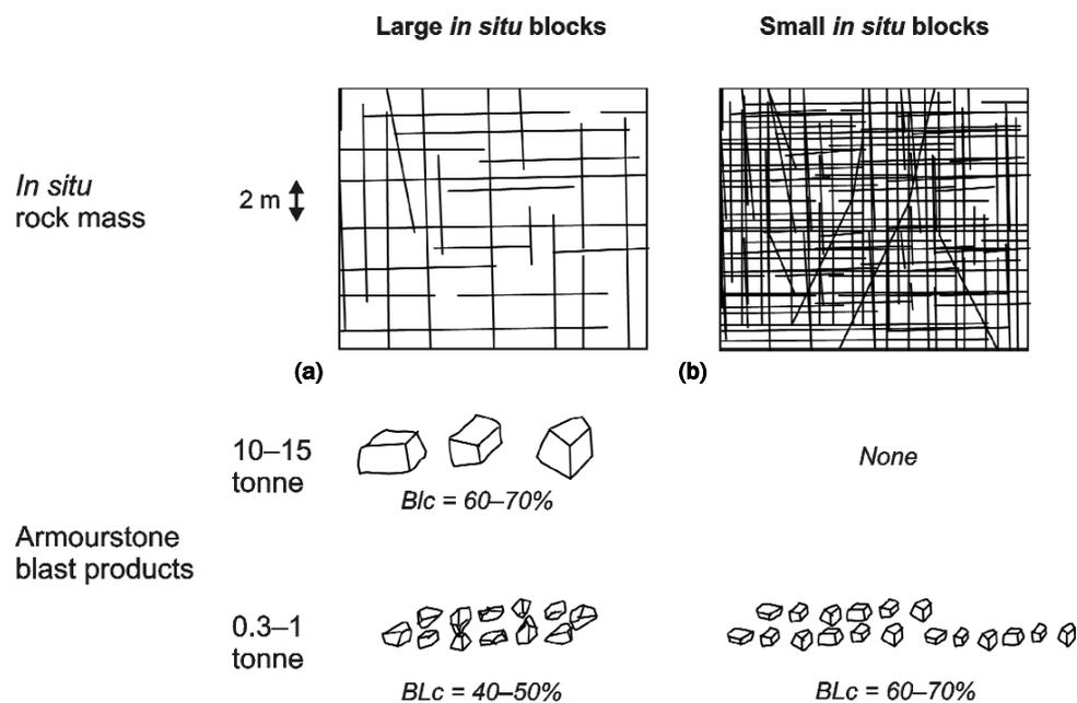
**Figure 3.18** Schematic illustration of the influence of discontinuity spacing and grading on the blockiness of armourstone in orthogonally jointed rock masses. Any spacing is possible; the 2 m spacing is an illustrative example (see text)
