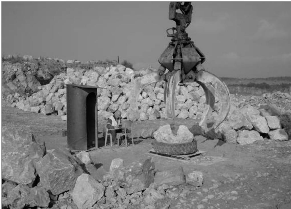
**Figure 3.81** Control testing of mass distributions of a 300–1000 kg standard grading during production using weighbeams (courtesy A Moiset). This set-up enabled 140 stones to be weighed per hour
